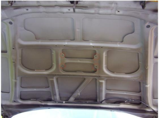
Now drill through the 4 holes circled using a drill bit smaller than the hole, so as not to fowl the edges of the hole. Try and keep an angle parallel to the hood. It is a good idea to place a blanket over the engine for the remainder of this project.
