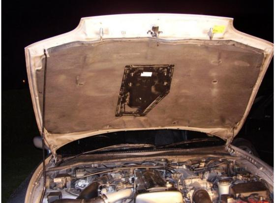
Now fully fit the under blanket back on the car except for the central 6 clips that have to hold the metal under air guide in place.
