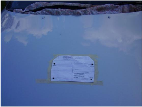
Apply masking tape around the template; lip it under the template for marking on.
