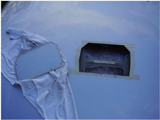
Now using a dremel cut along the felt tip line. You can sand the edge after if you wish but not essential, just cleaning.
