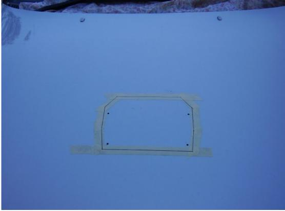
Draw around the template (on the masking tape) with a felt tip. Then remove the template and the screws.
