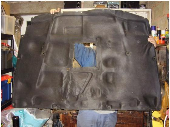
Now cut the hole in the under blanket using a knife.
