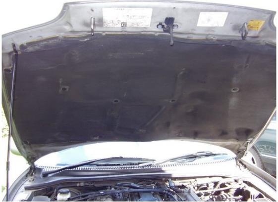
First remove the front rubber strip then the plastic clips, the centre rear 2 do not get removed as they are not the same as the rest and just hook onto a lip as apposed to through a hole.
