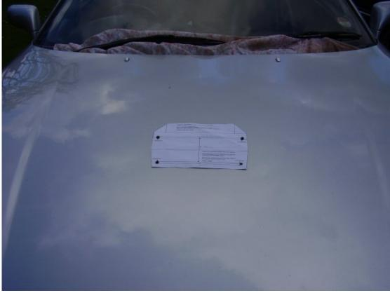
Now secure the printed template through the marked holes to the top of the hood. I used 4 screws that were to hand.
